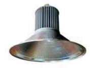
**Altitude:** Vertical design, LED Highbay luminaire with extruded aluminium heat sink having heat dissipating fins for larger surface area, satin finish powder coated in grey paint and fitted with multi-faceted anodised aluminium reflector.
