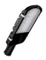
**Fiesta:** High efficiency, IP65 LED streetlight, with Power LEDs, aluminium pressure die cast housing, toughened glass in the front and peanut lens for batwing light distribution.
