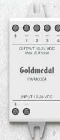
PWM0004 is a BLE-enabled four-channel PWM dimmer for constant voltage LED loads, such as LED strips and constant voltage LED modules. The same device can be used for both 12 and 24V DC LED strips. Separate drivers are not required for LED strip or RGB Strip dimming.
