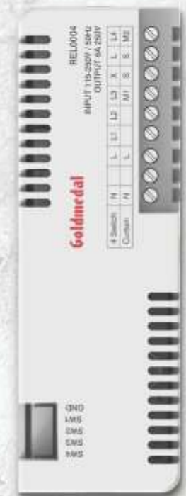
REL0004 is a BLE enabled 4 channel relay with 4 separate inputs to control BLE device on the network. The 4 inputs can be freely programmed to do operations like Dimming, curtains, master functions etc. The device can be used for curtain control also.
